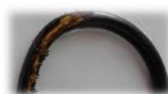
Exposed wiring of an electrical cord
