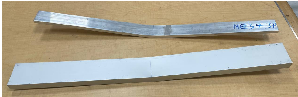
Figure 12. 3-Point Bending Test on Rectangular and Unreinforced C-Shape Cross-Section Beam
