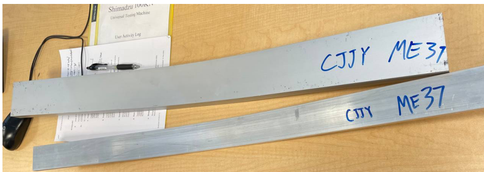
Figure 13. 4-Point Bending Test on Rectangular and Unreinforced C-Shape Cross-Section Beam
