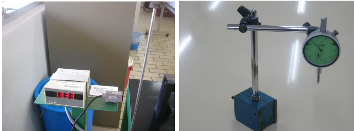
Figure 5 (a) Koyo Frequency tachometer (b) Dial indicator
